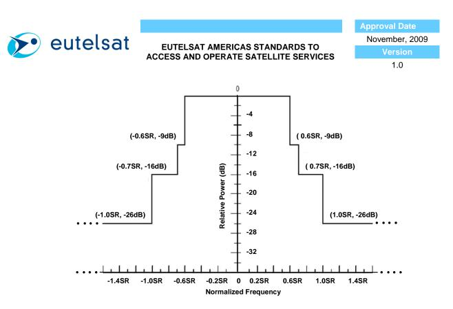
Figure 4. Mask based on the symbol rate, normalized to the center frequency of carrier
