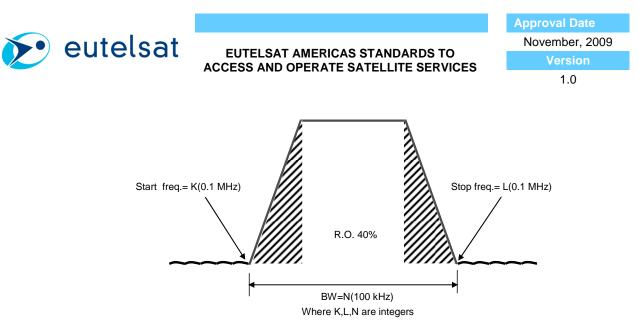
Figure 1. Banwidth for a single carrier per segment.
